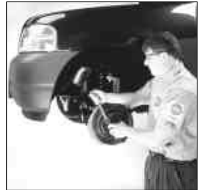
Step 1: Technician mounts an adapter to the hub.
