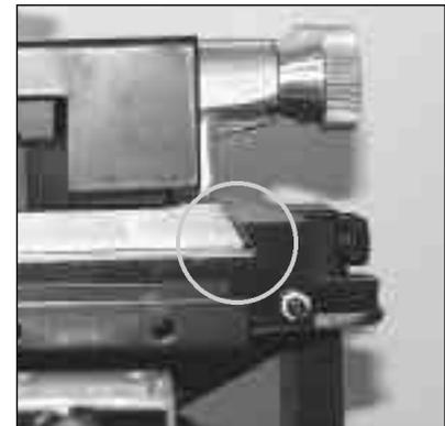
Note the dovetail at the back of the cutting head. This dovetail must be tight. Be sure to pull back on the cutting head as you secure the mounting bolt.
