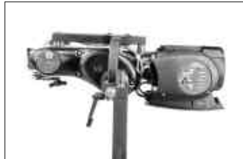
Lathe in upside-down position. You will need to flip the lathe over into this position to machine one side of the vehicle.
