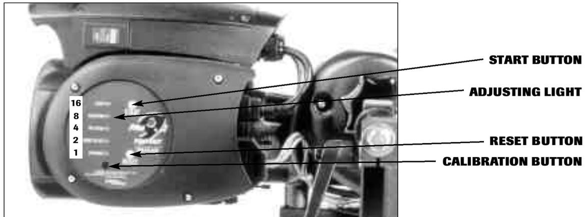
The illustration above shows binary values for each light. For example, when the 2nd and 4th lights are blinking, the total binary value is 10 (2 for light #2, plus 8 for light #4).
