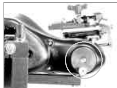
Move the cutting head by turning the knob shown above.
