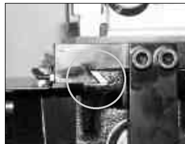
Detail of the gib that rides between the gear box and cutting plate.
