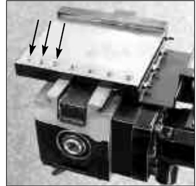
The cutting head connects to the cutting plate (50-498) by a bolt. The bolt threads through one of tapped holes in the plate. Different holes in the plate allow the cutting head to be set for any vehicle.
