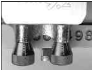
Turn the dials to advance the cutting head. Each line on the dial indicates 0.002”.
