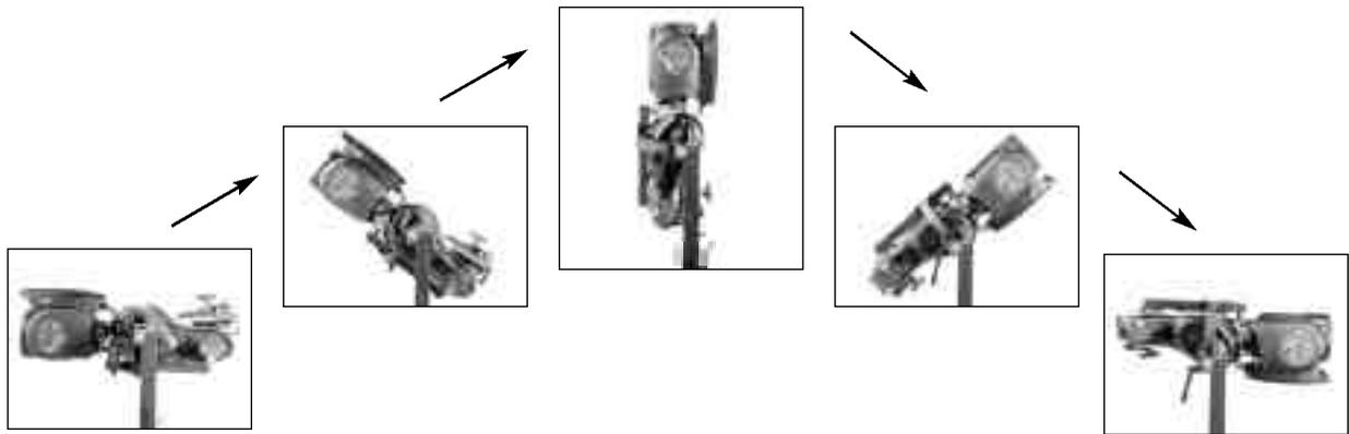
After loosening the trolley handle, the lathe can be flipped over to machine the opposite side of the vehicle.
