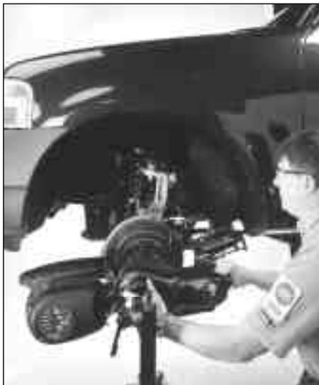
The PFM 9.2 On-Car Brake Lathe.
